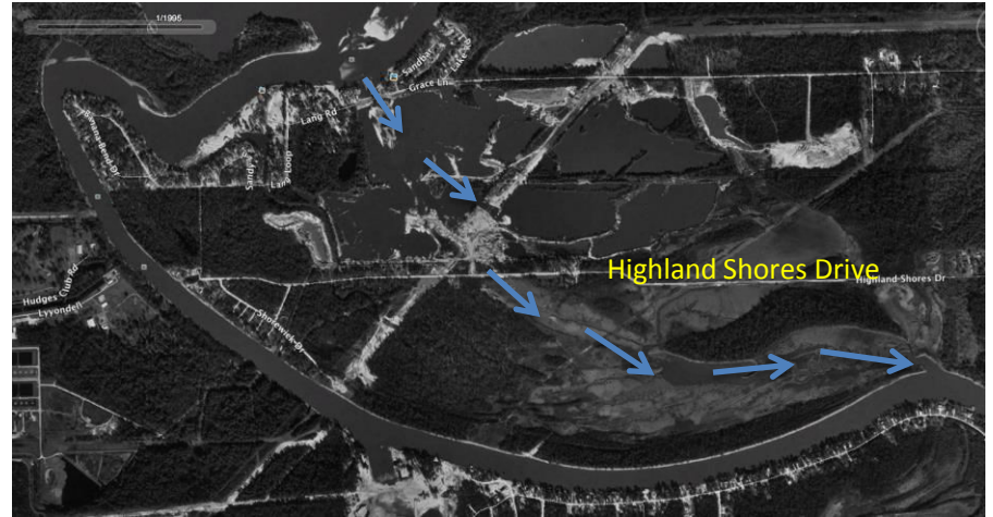
Banana Bend in 1995 after 1994 floodplain erosion. Evidently the flooded mine complex to the north of Highland Shores Dr connected with the channel to the south to provide a path for high flows across the floodplain. From Google Earth.
