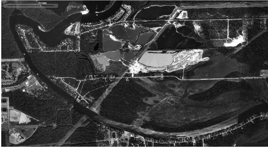
Banana Bend in 1989 before erosion of high flow channel in 1994 flood. Note sand mines in center of photo. From Google Earth.
